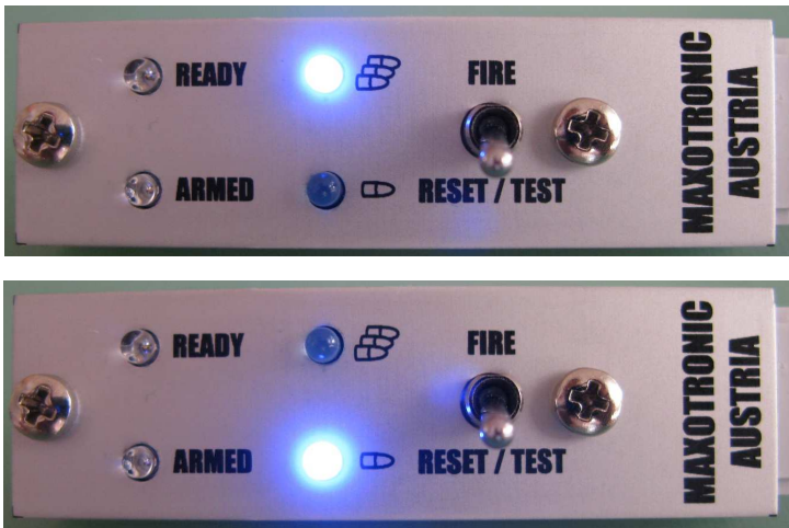
Fig. 2: Operation stages on the control unit during testing
