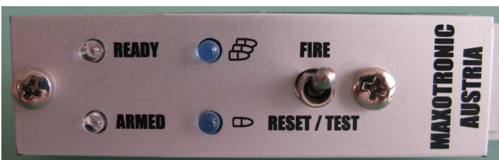
Figure 3: Control unit at position Fire
