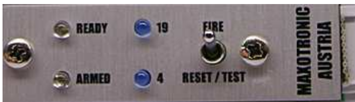
Figure 3: Control unit at position Fire
