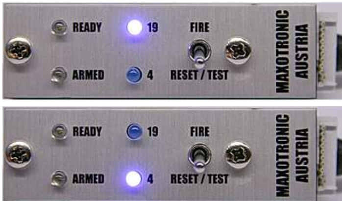
Fig. 2: Operation stages on the control unit during testing
